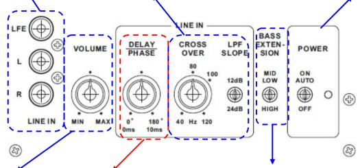
**Volume level setting** is determined by the efficiency of front speakers. It is not an indication of whether the sub can play louder or not.
