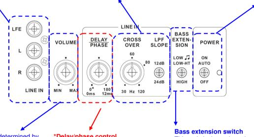
**Volume level setting** is determined by the efficiency of front speakers. It is not an indication of whether the sub can play louder or not.
