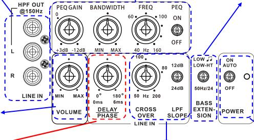
**Crossover setting** is a fine-tuning knob for integration. It is useful even when one already uses bass management. The upper end extension of the sub is limited to avoid using the servo subwoofer at frequencies where servo is less effective. Set to max by default. **LPF slope setting** determines the slope of crossover setting. For two-channel, one should use 24db whereas for HT input, one should use 12db.
