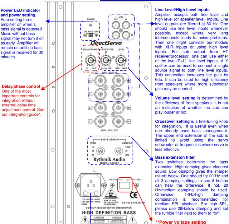
**Fuse box.** Use only correctly rated fuses. There is a notch to pry open the fuse box. Do not try to pull it off the amplifier. There are two fuses: the inner one is the in circuit fuse, and the outer one is a spare. Continuingly blowing fuses is an indication of a more serious problem. Contact us if this occurs.
